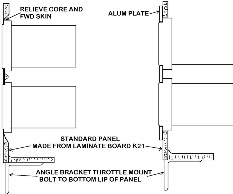
Switches are best grouped together. With the exception of the magneto and start switches all others can often go together in a line. The use of unitized switch/circuit breakers will simplify and improve your installation.
