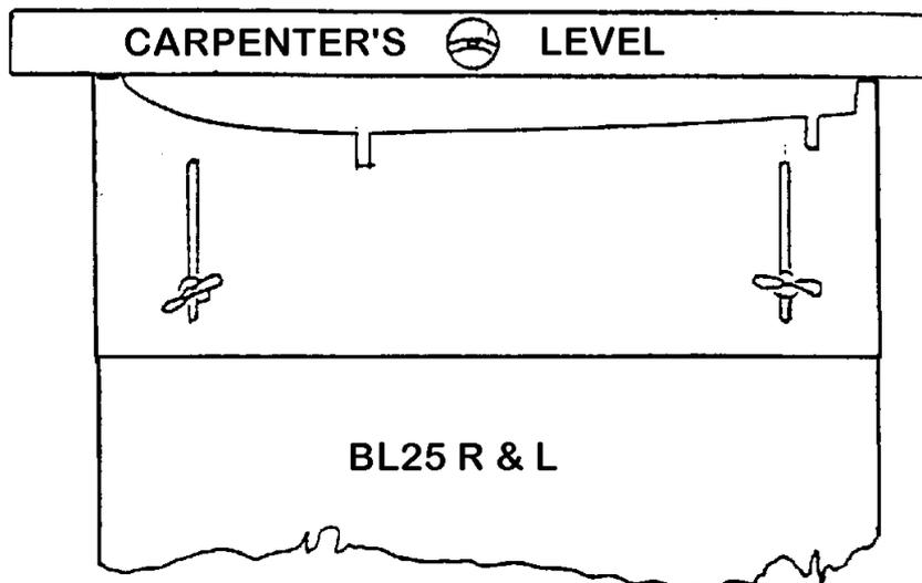
The BL118 jigs should be set approximately 4.1 inches below the BL25 jigs to allow for the 2½ degree dihedral. Set the exact cradle heights using the spar. Temporarily place the spar K117 in the cradles. Its face (web) should be oriented towards the leading edge; its proper position is approximately 13 inches behind the
