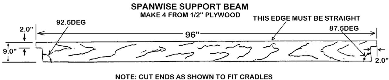
From the drawing you will note that each end of the two beams is relieved approximately 2 inches so that an indexing tab extends to assist in assembling the beams to the cradles. Exact dimensions can be determined by the builder by measuring the distance between cradle notches prior to cutting the beam ends. Note also that the exact angles of the ends may best be cut about  $2\frac{1}{2}$  degrees off perpendicular to allow for the dihedral angle in the cradle jig set-up.
