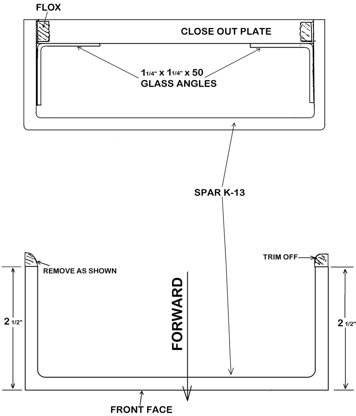
Locate the spar close-out plate K15, it is a prefabricated composite approximately 0.40 by 6 by 50 inches. Locate and mark the two hardpoints in the plate. Locate the two fiberglass angle brackets K116, they are 1¼ by 1¼ by 50. The angles and close-out plate will be accurately centered and bonded into the spar.
