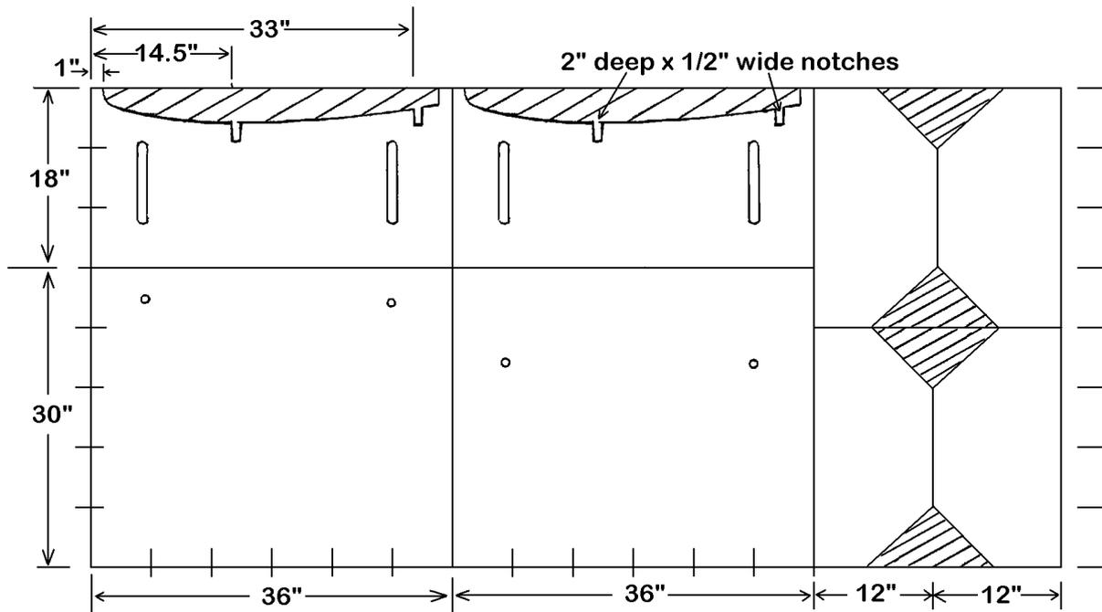
Find space in the shop where the basic wing can be assembled less tips. The size less tips is 4 by 20 feet. Pluck a span-wise chalk line on the floor. Mark Center Line, BL25 left, BL25 right, BL118 left, and BL118 right. Set up the four cradles perpendicular to the span-wise line on the BL25 and BL118 marks. Set the cradles at the same approximate height (such as full down) and level each with a long carpenter's level or a
