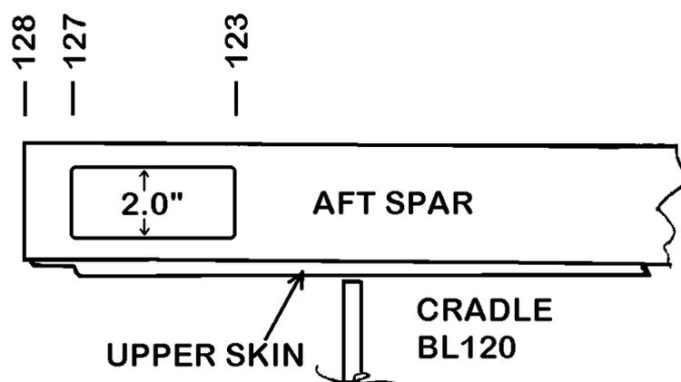
Measure aft  $1\frac{3}{4}$  inches from the aft spar and mark a line on the upper skin. It should go from the root at BL19.5 to the tip at BL128.0. Trim the skin slightly behind this line and block sand to the exact line. Further trim the skin so that it is flush with the aft spar from BL19.5 to BL25.
