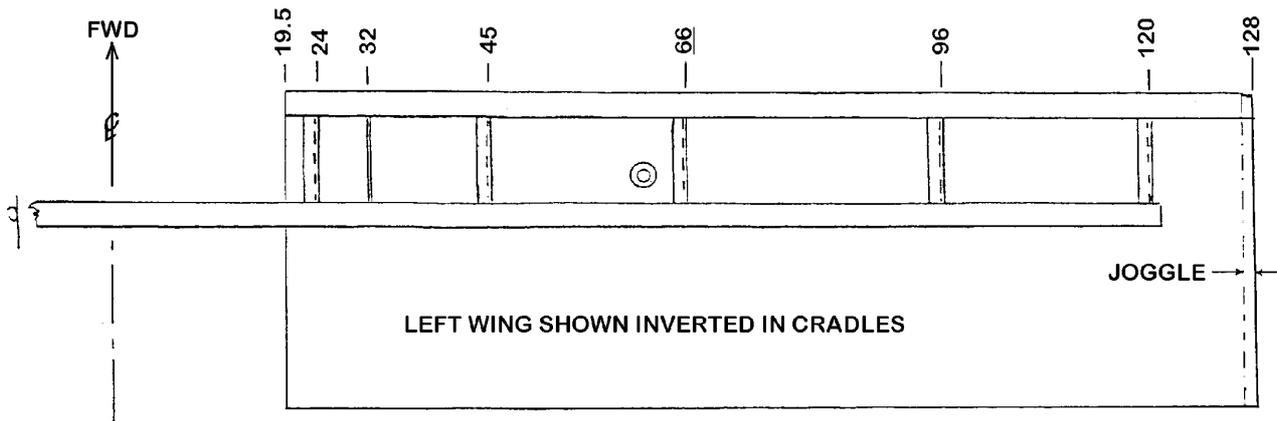
Remove the spar and ribs but keep all the weight and clamps handy because they will be needed for the actual gluing operation. Sand all the contact areas of the skin, ribs and spar with 80 grit sandpaper in preparation for bonding.
