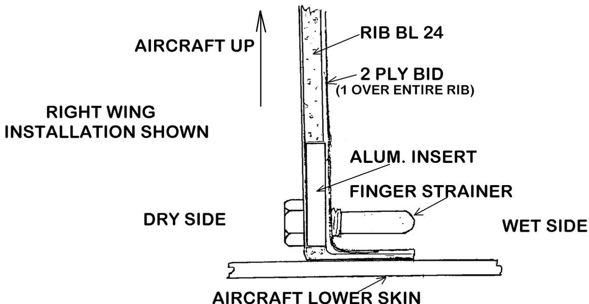
Don't forget that both ribs have the lip on the right side. After the 3/8 pipe tap operation, check that the finger filters install satisfactorily. Remove them and put just a little hard wax or modeling clay into the phenolic threads to keep them clean until the filters are permanently installed at a later time.
