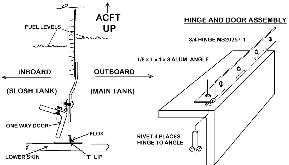
There is one structural rib located in each tank at BL45. Take two factory preformed ribs and make holes as shown in the sketch. Dremel and router bits are good for this. Don't worry about removing a small amount of flange.
