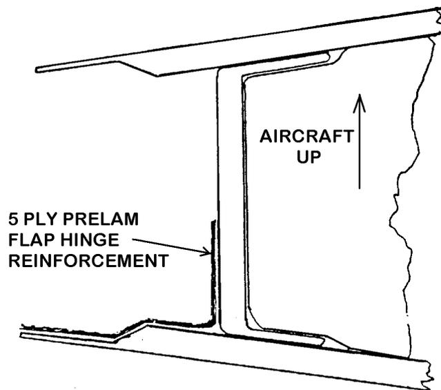
Relieve the upper skin trailing edge by  $\frac{3}{32}$  inch where the aileron hinges are installed just as you did when you built the stabilizer and elevator. In a similar manner relieve the lower skin for the flap outboard and center hinges. Install eight hinges, four aileron and four flap, with #8 c.s. screws, Tinnerman washers, and elastic stop nuts.
