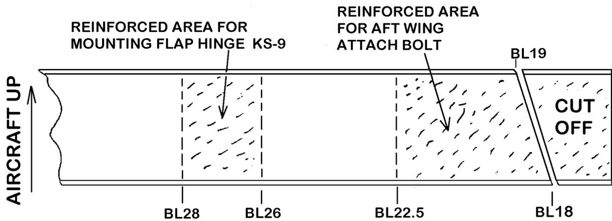
When installed the aft spars must be properly spaced out from aircraft center line. The pointed ends are to be at BL19R & 19L. This makes the ends 38 inches apart. The outboard end of each will extend a little beyond the end of the skin.
