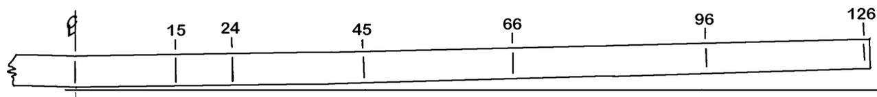
Using a bright light behind the spar web, find the aluminum reinforcement plates that are centered at approximately BL15 left and right. Mark their location in the spar structure. These are the main attach points for the wing. During assembly of the wing to the fuselage you will be required to drill through these blocks and be near to their centers. If you find that the centers are not within plus or minus  $\frac{3}{4}$  inch of BL15 call the factory for instructions.
