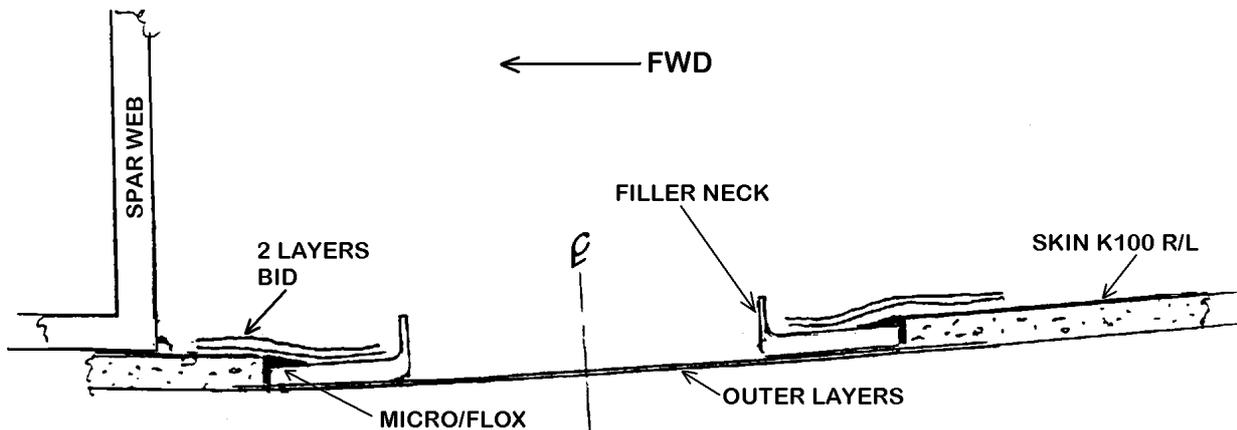
The next step involves making two slosh compartment ribs. These will be located at BL 32R & L. Their purpose is to assure that there is always fuel available at the tank outlets to feed the engine regardless of lateral sloshing. Each slosh rib will have a one-way door installed at the bottom that will allow fuel to flow only towards the center of the airplane and be trapped where it can feed the engine.
