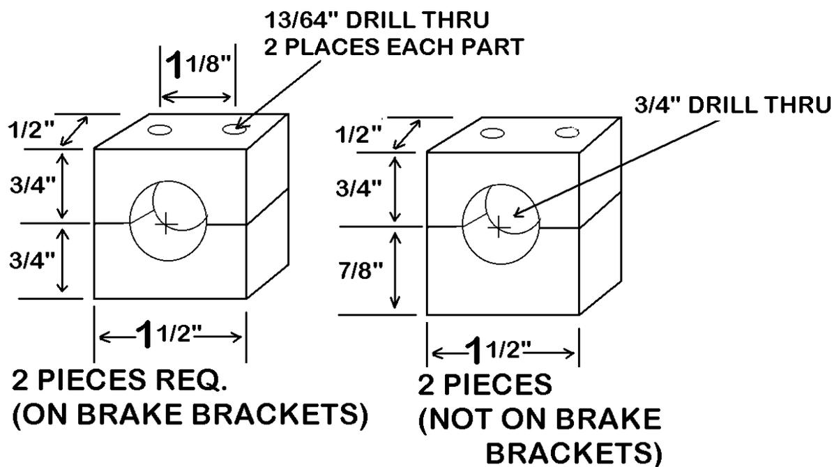
**FIGURE -Mounting blocks for rudder pedal assembly**
