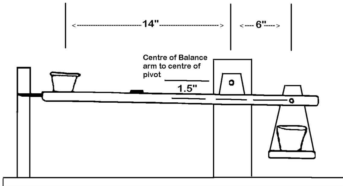
The perspective view in the next figure shows how the balance is set up for use. The main ballast weight is to balance out the unequal arms of the lever, and if you use the same type of containers all the time it can be glued in place for convenience. Set up balancing for each use can then be accomplished by moving the smaller ballast weight. Verify the accuracy of your construction by using quantities of small uniform items
